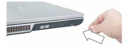
**10** Carefully slide the drive out of the drive bay.
